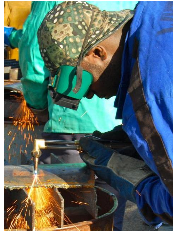
Apprentice practicing cutting steel wearing protective gloves and welding goggles. (Neil Libby/CPWR/elcosh.org)
