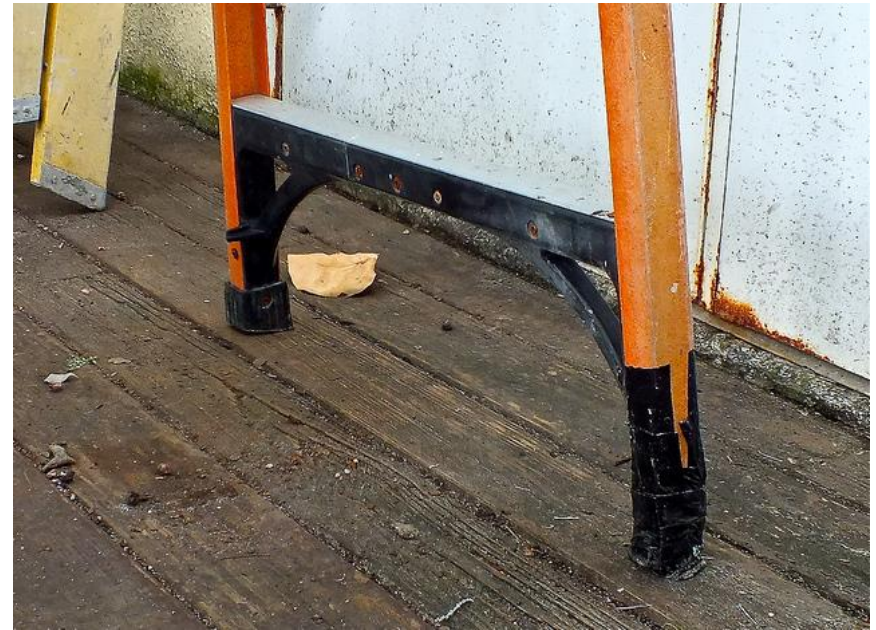
Damaged footpad/assembly on this step ladder was poorly taped over in a bad attempt to fix the ladder. (*2)
