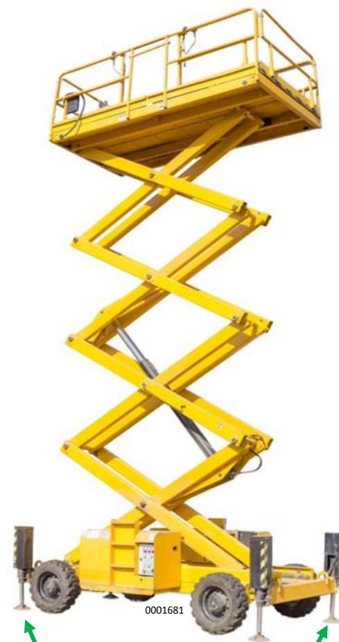
Outriggers used to stabilize and level the scissor lift.
